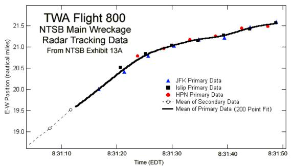
**Figure 1:** Radar data that represents the east-component of main wreckage flight path. The solid black line is a 200-point cubic spline interpolation of the mean of all of the primary radar data representing Flight 800's main wreckage in NTSB Exhibit 13A.
