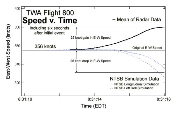
**Figure 2:** East-West Speed vs. Time plot comparing the radar data with NTSB simulations. The NTSB simulation data shown is a time differential of the East-West position data in NTSB Exhibit 22C. An offset of 24 knots was added to the NTSB data after differentiating to align with the radar data. The radar speed data was differentiated from an interpolation of the mean of the "main wreckage flight path" radar data in NTSB Exhibit 13A.
