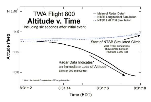
**Figure 3:** Altitude vs. Time plot comparing the radar data with NTSB simulations. The NTSB simulation data shown is from NTSB Exhibit 22C. The Law of Conservation of Energy was applied to the speed data in Figure 2 to calculate the loss of altitude (see discussion below).
