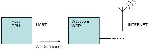
**Multiplexing:** Several sockets can be operating at once. The +WIPDATA command allows to temporarily identify the UART in data mode with a given socket. The data written on UART is transferred through the socket. The data which arrives on the socket can be read from the UART. In AT mode, the host receives an unsolicited event when the data arrives on the socket.
