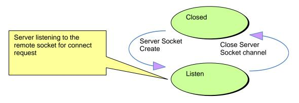
On reception of a connection request from a remote client socket, a server socket does the following:
